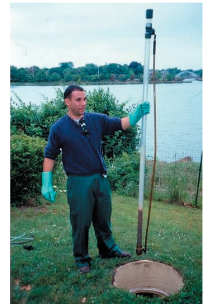
Inspection is a fundamental part of maintenance. This device measures scum and sludge depth in the septic tank.
