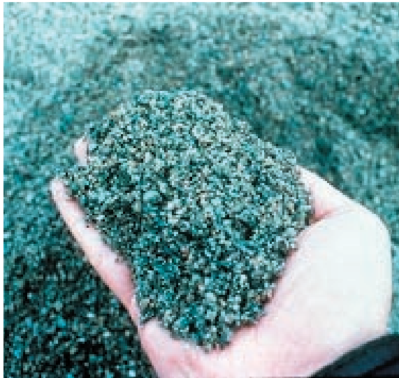
The uniform, specified grain size of the sand used in a Wisconsin Mound (above) is required to enhance wastewater treatment. "Bank run" gravel (below) is often used in other fill systems. The coarse fragments and stones provide little surface area for physical or microbiological treatment in the fill type drainfield.
