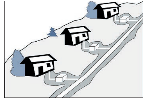
Septic Tank Effluent Collection. Graphics: NSFC.
