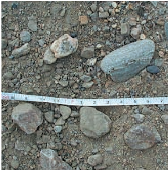
The uniform, specified grain size of the sand used in a Wisconsin Mound (above) is required to enhance wastewater treatment. "Bank run" gravel (below) is often used in other fill systems. The coarse fragments and stones provide little surface area for physical or microbiological treatment in the fill type drainfield.
